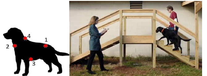
Fig. 1. Diagram showing the sensor locations. The platform used to measure dynamic activities [7].
